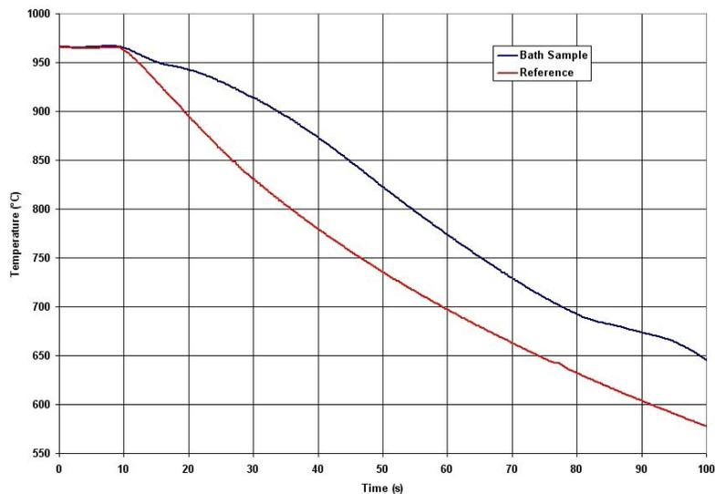
Figure 3: Recorded cooling rate of bath sample and the metallic mass of the probe, which act as reference temperatures in the DTA
