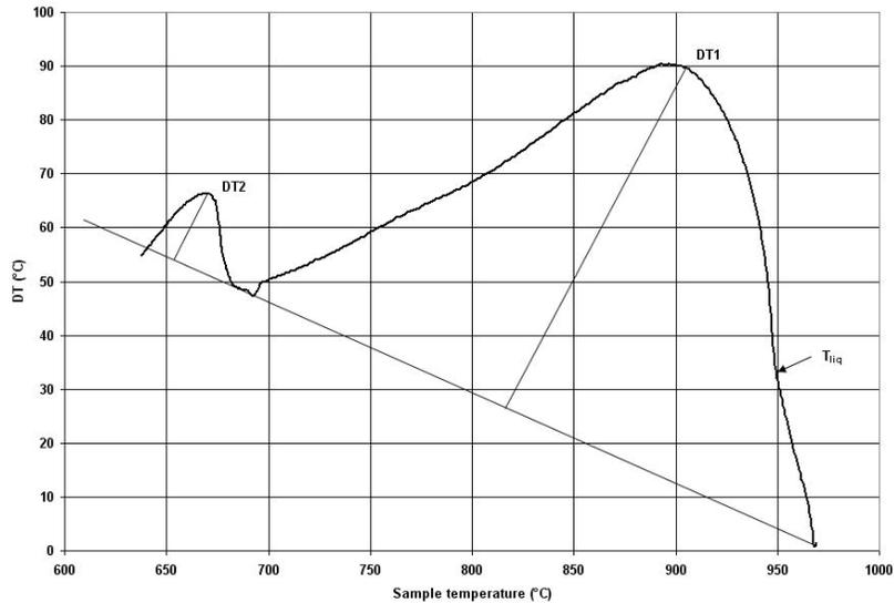
Figure 4: Differential temperature curve and one possible way to perform the DTA analysis
